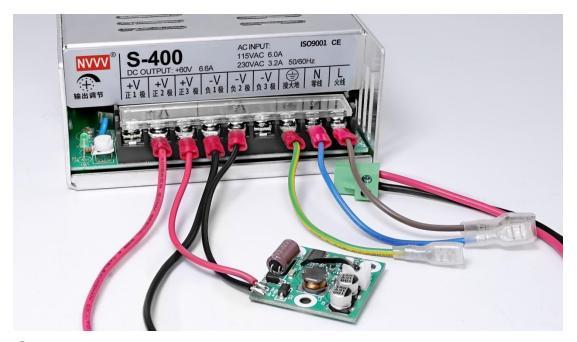
(5) Install the switch power supply
